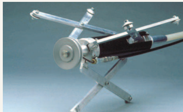
Orbiter III suits pipes from 7 inches to 37 inches.
