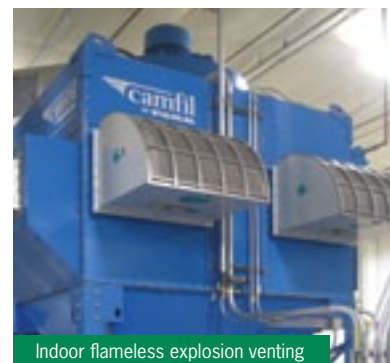
Indoor flameless explosion venting
