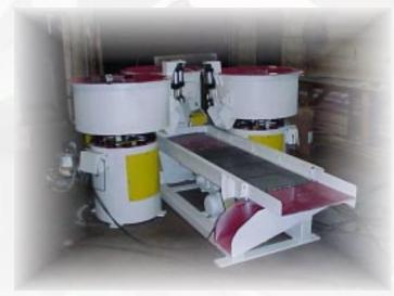
Multiple process bowls feeding a common screen deck. Unique solution engineered systems like this are what separate Giant from the rest.
